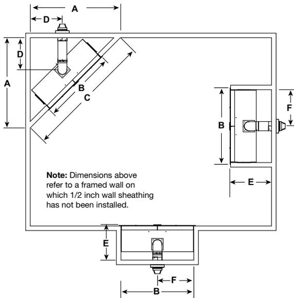
The rough framing dimensions shown represent the distance from stud to stud only and do not take into consideration the addition of drywall. Please refer to installation instructions for complete specifications and drawings when installing this product. Go to [heatilator.com](http://heatilator.com) to download.
