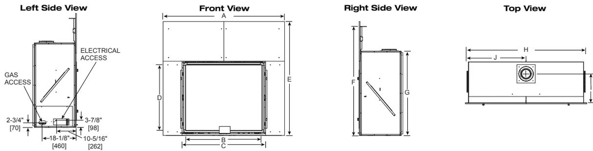
\*Front dimensions include non-combustible material which overlaps framing
